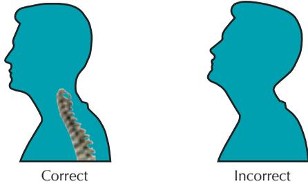
Eliminate work done at slight flexion. To avoid this posture, the height of the work area may be raised.
